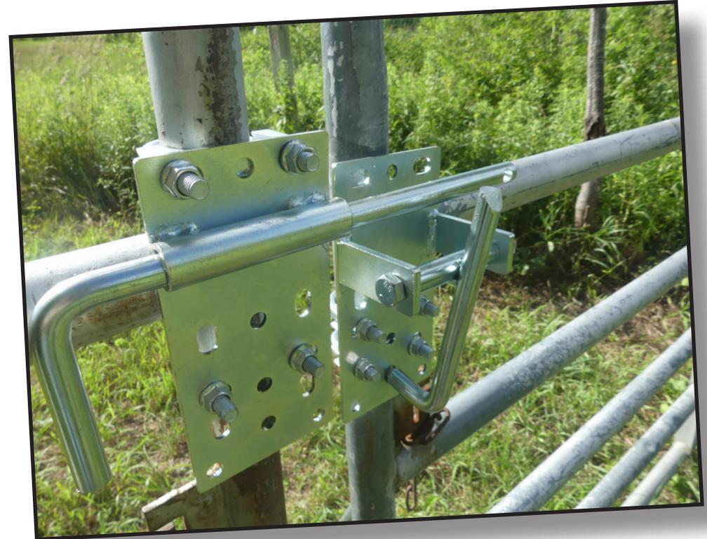
At Tech Team we make several different types of latches for farm and cattle gates and one of them is going to work best for your gate. Our automatic trip latch allows you to swing the gate closed and then automatically latches. No bolts to slide or handles to pull. To disengage the latch you can either slide the bolt back or toggle the pendulum.
