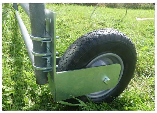
The Tech Team\* #768 Heavy Duty Gate Wheel will support up to 400 lbs. and is designed primarily for tubular steel agricultural gates but can also be used for wood gates and cyclone fence style gates. The flat free tire and 16" diameter make it the perfect choice for large heavy gates and it can easily negotiate uneven surfaces and turf.
