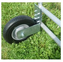
Final Steps - Once the bracket has been securely put in place, elevate the gate a little bit, put the wheel on, refasten the castle nut, insert and spread the cotter pin, and the job is finished
