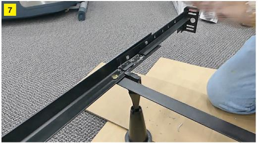
One nut and screw can work if the headboard is supported on the floor, however 2 screws makes a much better job.
