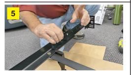
With the extension set to at least 80" align the holes in the bracket with the holes in the frame and attach with one screw and nut. If another set of holes lines up use another screw and nut, if not see the next step.
