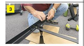
The opening in the bracket is designed to fit over the rivet that attaches the cross member.
