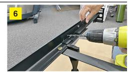
Use one of the holes as a guide then use a drill and a 1/4" high speed bit to make another hole and attach with a screw and nut.
