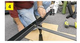
Sometimes the bracket needs to be mounted ahead of the rivet so that the finished extension is at least 80". Remember, all bed frames may not be identical.
