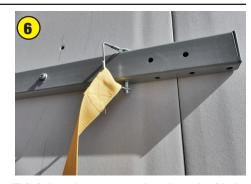
This is how the straps attach to the rack with the PTO Clips.
