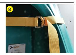
This shows how the straps engage the D rings to secure the boat in place.
