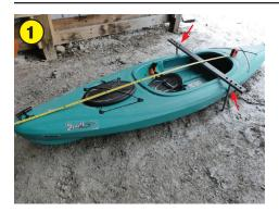
Thread the threaded rods into the member with the threaded holes. You can select any of the holes that will be appropriate for the width of your boat. Once you've threaded the rods in, put it over the boat to see where it fits best, and then measure from the bottom end of the boat to the rack, and this will be the height that you anchor this particular member.
