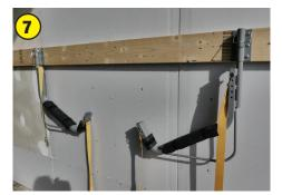
Hook folded flat against the wall. Align the correct holes in the hinge and the hook shank. Secure with the PTO clip.
