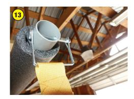
Now attach the straps with the plain end to the ends of the 4 arms using a PTO clip as shown.
