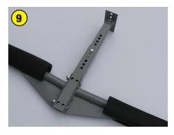
The support arms mount to the extension part of the bracket, using the 4 holes in the lower portion. Using 4 x 75mm M12 bolts and nuts, fasten two arms opposed to each other as shown.
