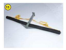
This is how the assembled extension pieces and arms will appear. The arms angle upwards at a 3° angle to ease the boat towards the center.
