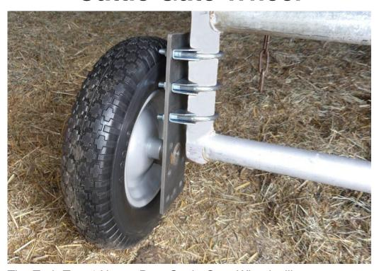
The Tech Team® Heavy Duty Cattle Gate Wheel will support up to 400 lbs. and is designed primarily for tubular steel agricultural gates but can also be used for wood gates, sliding gates, and cyclone fence style gates. The flat free tire and 16" diameter make it the perfect choice for large heavy gates and can easily negotiate uneven surfaces and turf.
