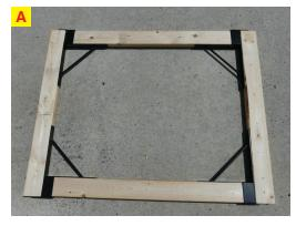
Measure the opening for your gate. The gate we are When positioning the corner brackets, it is suggested illustrating is 36" wide x 48" high but this is for the to move them 2"-4" from the bottom and top edges purpose of illustration only. Using fascia boards ( $\frac{3}{4}$ " x of the gate as shown. (See #1) This allows sufficient 6" would be appropriate) position the corner brackets overhang so that the top and bottom edges can be as shown.
